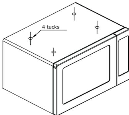
Fasten the oven with screws and washers.
